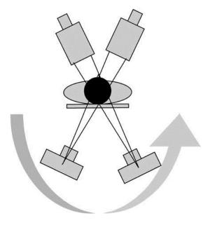
\*\*\*Effect of dose spreading by varying the beam incidence angle. The maximum dose thus tends to be spread over a broader area of the patient's skin.\*\*\*
