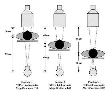
\*\*\*Effect of geometric magnification on entrance skin dose. With fixed source-to-image receptor distance, both magnification and skin entrance exposure (SEE) increase as the patient is moved closer to the x-ray source.\*\*\*
